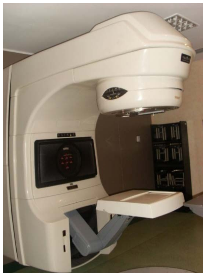
Fig. 2: "Clinac 2100c" linear accelerator used irradiation of the sugar samples.
